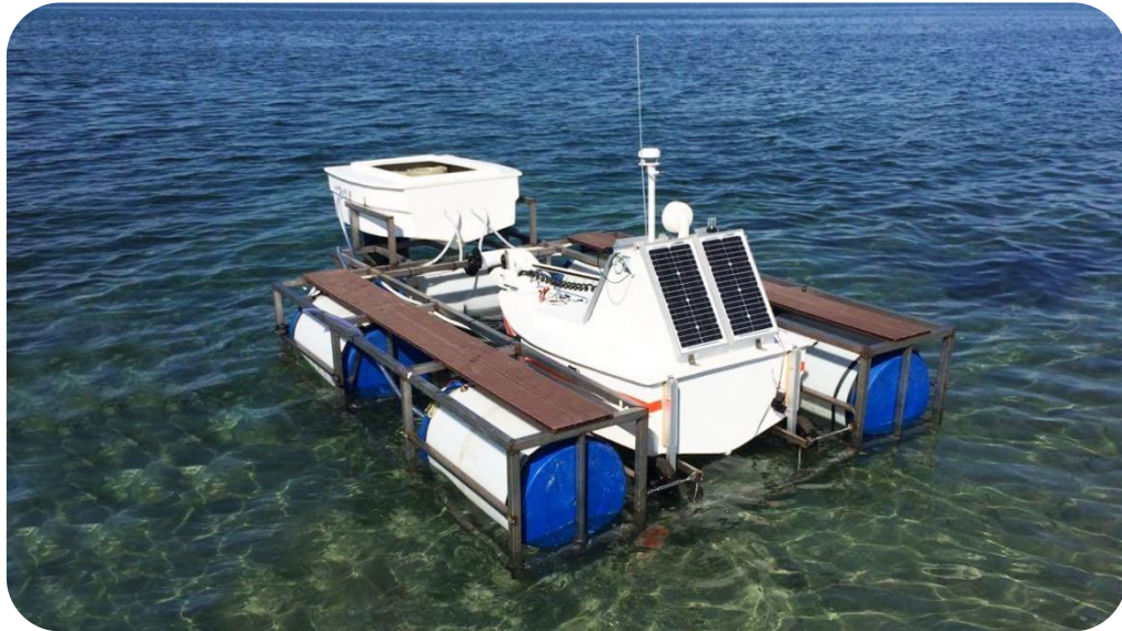
The Automated Floating Mechanism is the Docking Station of the AWTSS-1
